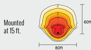
All published photometric testing performed to IESNA LM-79-08 standards by a NVLAP certified laboratory. Fixture photometry was completed on a single representative fixture.
