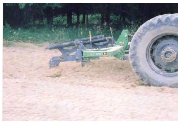
Fig. 11. A repeat run of the 3-shank ripper along the same patterned pass area as Fig. 9; here, incrementally reaching 18 of the needed 22 inches of subsoil fracture.
