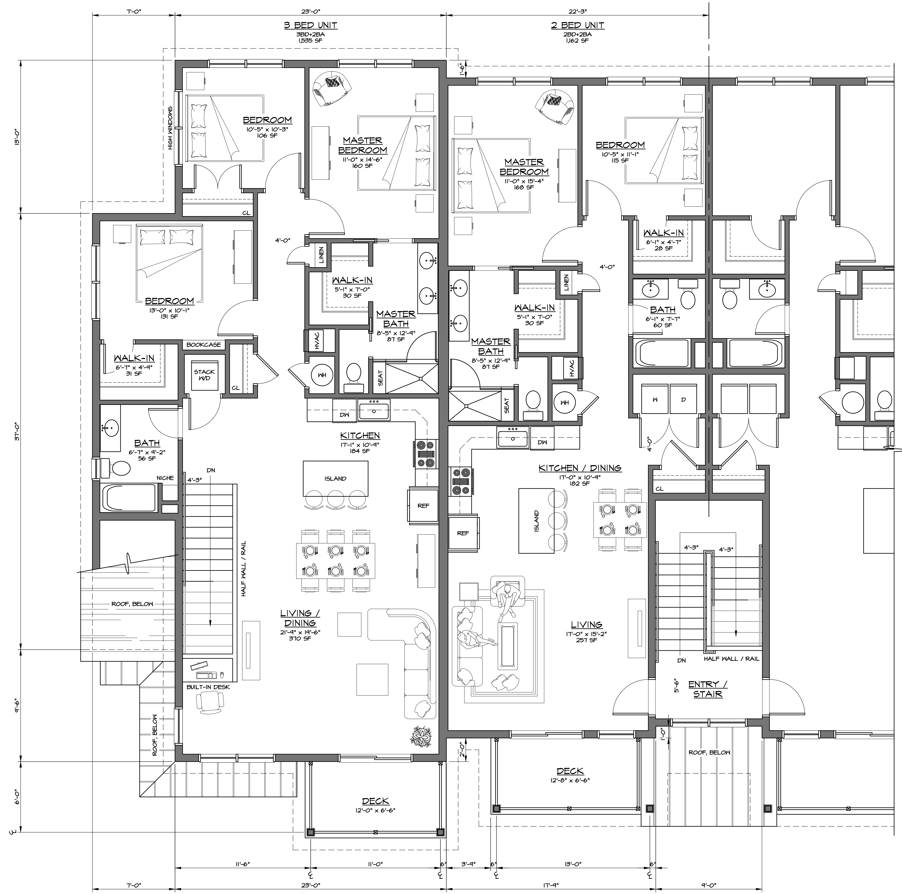
1 2 TYPICAL UNIT PLANS - SECOND FLOOR
