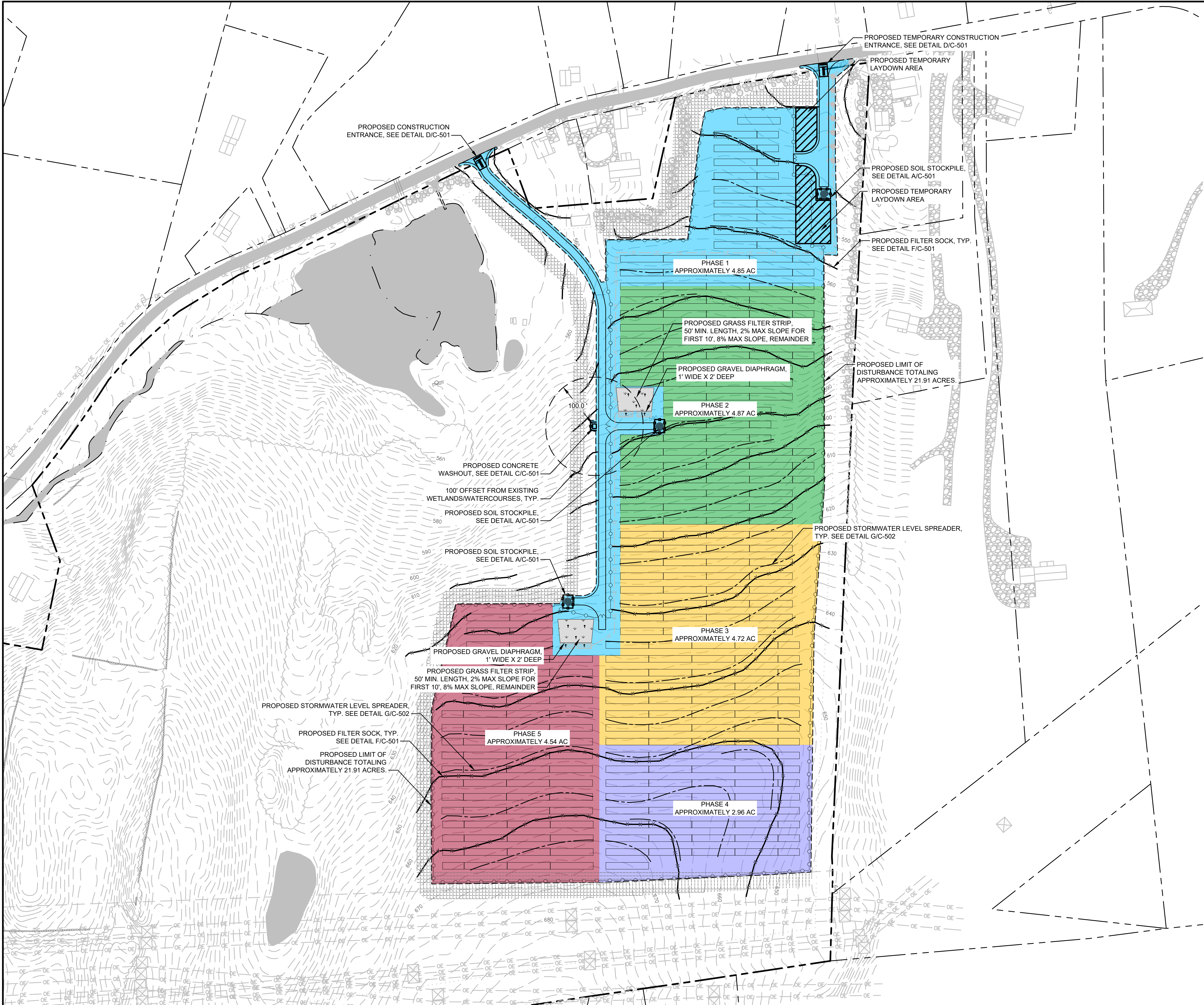
PROPOSED EROSION & SEDIMENT CONTROL PLAN SCALE: 1"=100'
