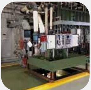
S&L pump stations are factory-built and assembled, and tested to Hydraulic Institute standards in state-of-the-art facilities that replicate actual field conditions. Our customers are invited to witness testing at our factory.
